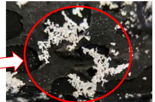
Fig.1 Deposit silver from a bamboo charcoal
