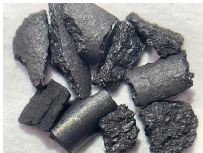
Fig. 2 The carbon rod soaked in \text{AgNO}_3 aq
