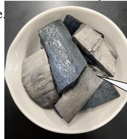
Fig. 7 bamboo charcoals and metals deposited on charcoals
